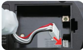
Remove the battery pack from the Meniett package. Plug the white four pin connector on the battery pack into the mating connector in the Meniett device, pushing downwards until fully seated. NOTE: Make certain that the tabs and slots on the two connectors are aligned.
